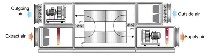
Figure 3. Frost protection with preheating of extract air.
