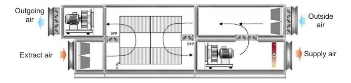
Figure 4. Frost protection with recirculation.
