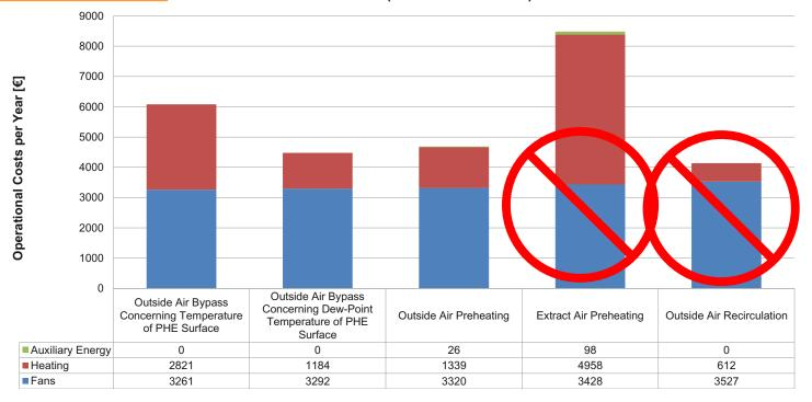
**Figure 5.** The operational cost (heat and electricity) of frost protection in the case study with an air handling unit of 4 000 m<sup>3</sup>/h.
