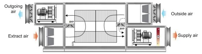
Figure 1. Frost protection by ourdoor air bypass.
