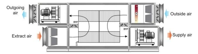
Figure 2. Frost protection with preheating of outdoor air.
