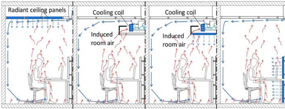
**Figure 1.** Operating principle of the four cooling systems (from left): radiant ceiling (CCMV), chilled beam (CB), chilled beam with radiant panel (CBR) and mounted local radiant cooling panels with mixing ventilation MVRC. Note: Only half of the room is shown with symmetry line on right side.
