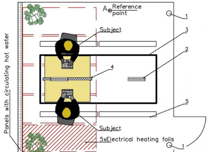
**Figure 2.** A) Top view of the test room with measurement pole locations: 1) ventilation exhaust, 2) ventilation supply, 3) chilled beam (CB), 4) desk partition mounted radiant cooling panels, 5) light fixtures, B) photograph of the measurement setup in CB, CBR and CCMV cases and C) photograph of the measurement setup in MVRC case (thermal mannequins above were used in actual measurements).
