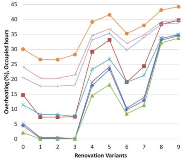
**Figure 2.** Percentage of overheating hours (measured only for occupied hours) for different renovation variants (Table 2) in room level for both methods of assessment, for the southern French case study.
