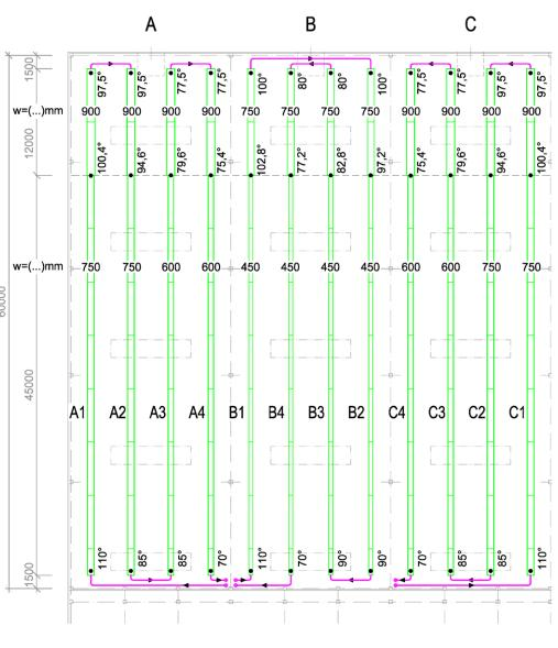
Figure 2. Optimal location and connection of radiant strips.
