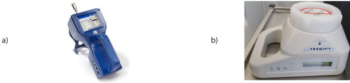
**Figure 3.** Measurement instruments, a) AEROTRAK™ Handheld Particle Counter Model 9306, b) CFU measurement device.
