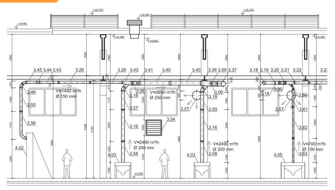
Figure 3. Local exhaust equipment – Cross section of wood industrial facility hall. [13]
