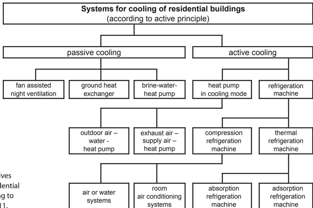
**Figure 1.** Alternatives for cooling of residential buildings according to DIN V 18599-6: 2011.
