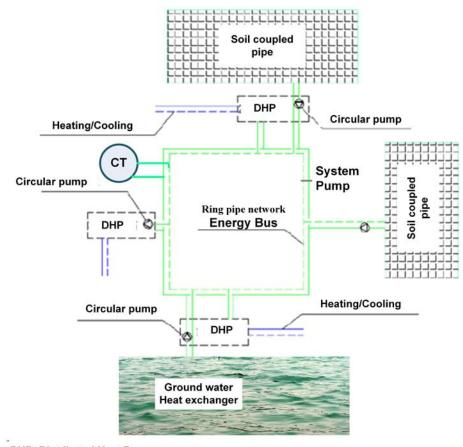
DHP: Distributed Heat Pump CT: Cooling Tower
