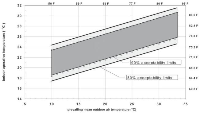
Figure 1. Acceptable operative temperature ranges for naturally conditioned spaces. Source: ASHRAE 55 (2013).
