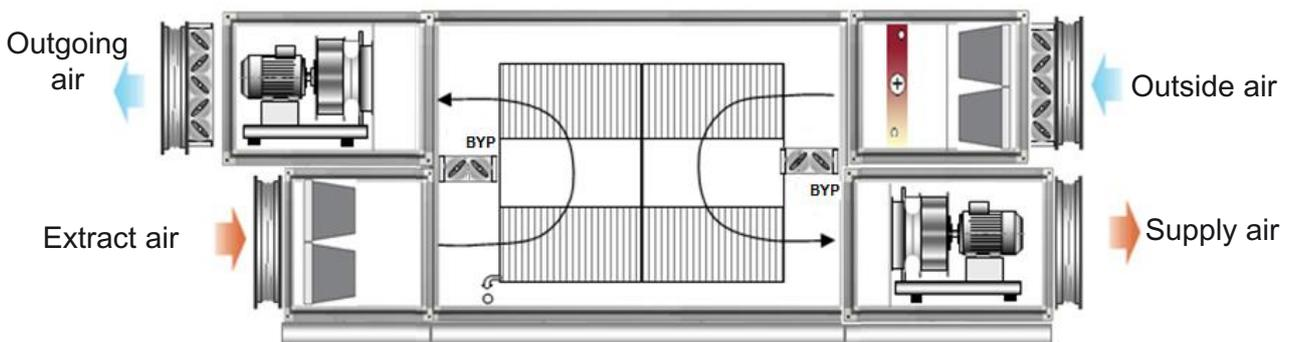
**Figure 2.** Frost protection with preheating of outdoor air.
