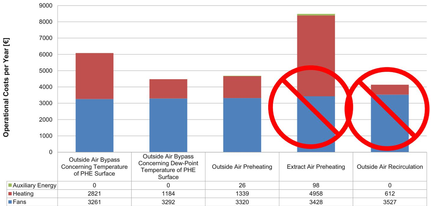
**Figure 5.** The operational cost (heat and electricity) of frost protection in the case study with an air handling unit of 4 000 m<sup>3</sup>/h.
