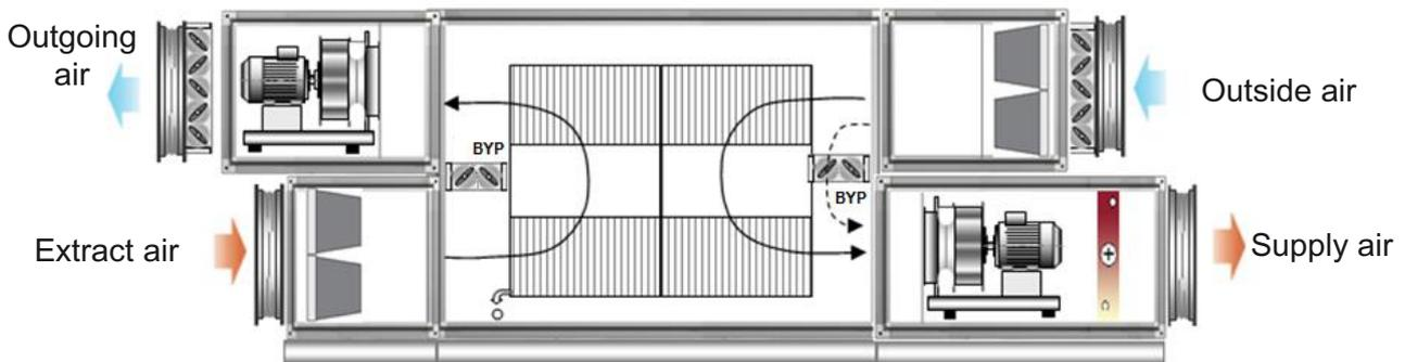
**Figure 1.** Frost protection by outdoor air bypass.
