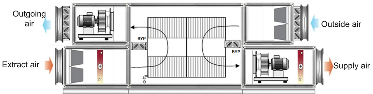
Figure 3. Frost protection with preheating of extract air.
