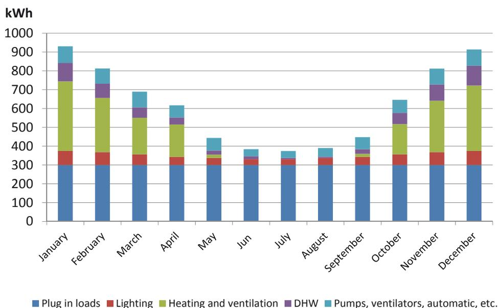
Figure 3. Break down of building electricity consumption by month.
