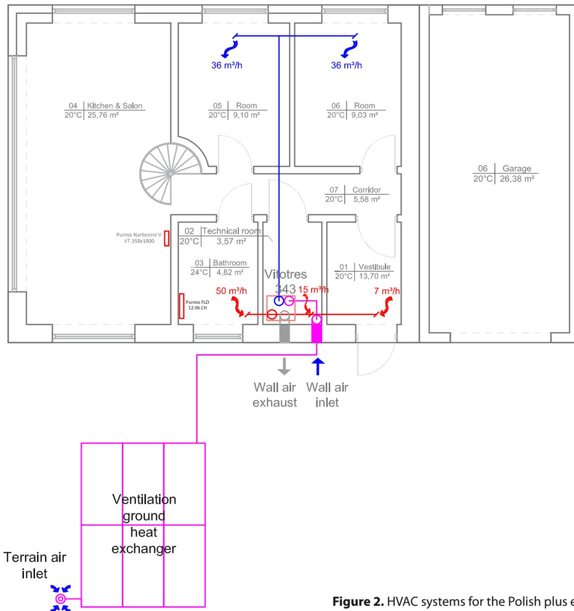
**Figure 2.** HVAC systems for the Polish plus energy house.
