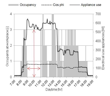
**Figure 10.** Occupancy for 4 workplaces and total energy demand for those places for a reference day, time step = 5 minutes. The red arrows indicate that energy demand can be reduced when the occupants are not at their workplace.
