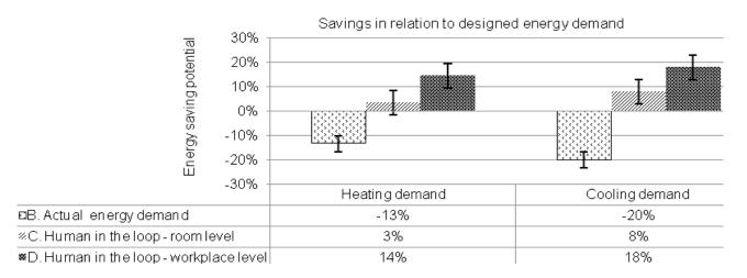
**Figure 11.** Energy savings compared to designed energy demand for actual energy demand (B), energy control on room level (C) and sending energy to the individual on workplace level (D).
