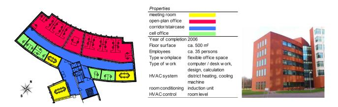
**Figure 4.** Floor plan of the case study floor (A) with the important properties of the floor (B) and a picture of the building from the outside (C).
