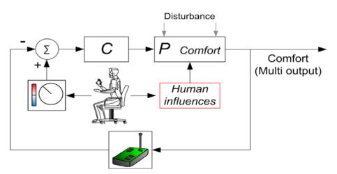
**Figure 3.** Proposed block diagram of the controlled system with the intelligent coordinator to take the human influences in the loop of building systems via feed forward control.
