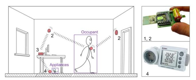
**Figure 5.** A wireless sensor network (2) tracks the mobile node (1) of the occupant and the energy use of appliances (4) and uses the real-time data for the building system control (3).
