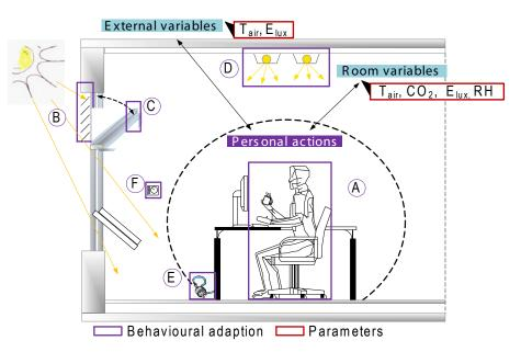
**Figure 1.** Parameters for human comfort (red box), with the user actions to influence the environment, B. blind control, C. window opening, D. lighting – and F. thermostat control (purple box) and user influence influencing indoor environment, A. user presence and E. use of appliances (green box).
