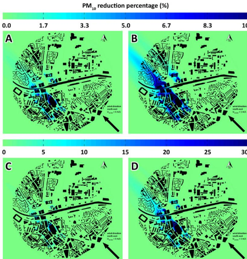
**Figure 4.** Contours of  $\text{PM}_{10}$  concentration reduction percentage at a height of 1.75 m for the case with 99 units (a, c) and 594 units (b, d) relative to the reference case without units. Wind direction South-East  $U_{\text{ref},10\text{m}} = 1 \text{ m/s}$ . [3]
