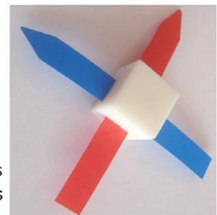
**Figure 2.** Same examples of the heat exchangers produced by additive manufacturing.
