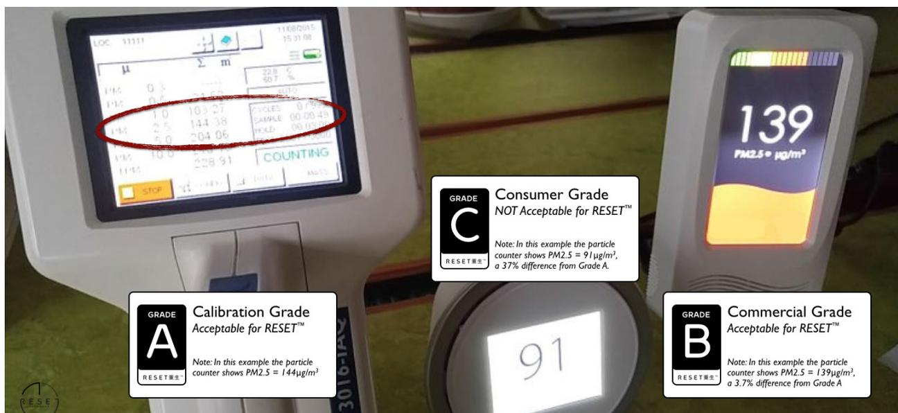
**Figure 4.** Varying accuracy of three monitors show the difference between monitor quality grades. General rule: if you can’t calibrate it, don’t buy it. Only Grade A and Grade B monitors are accepted for RESET™. Latest RESET™ standards are here: [http://reset.build/resources/RESET\\_Accredited\\_Air\\_Monitor\\_Requirements](http://reset.build/resources/RESET_Accredited_Air_Monitor_Requirements)
