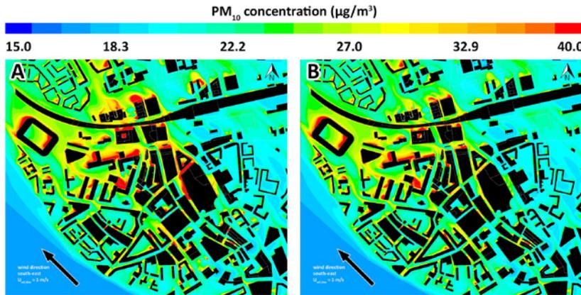
**Figure 3.** Contours of  $\text{PM}_{10}$  concentrations ( $\mu\text{g}/\text{m}^3$ ) in a horizontal plane at 1.75 m height without units (a) and including 594 units (b) installed over 16 parking garages in the city center of Eindhoven. Wind direction South-East  $U_{\text{ref},10\text{m}} = 1 \text{ m/s}$ .
