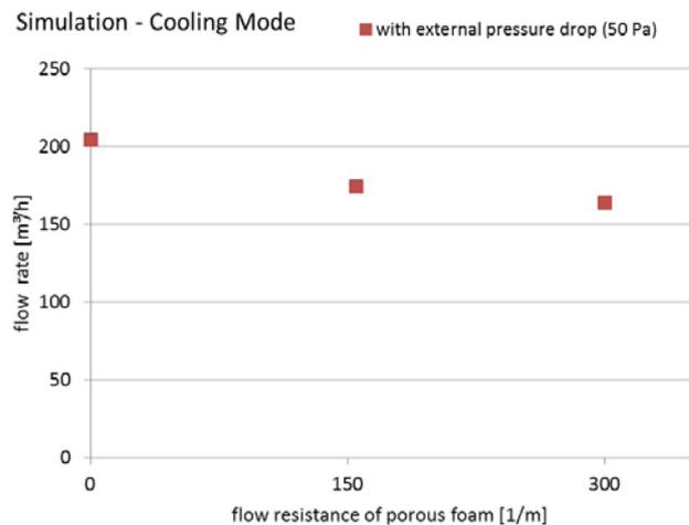
**Figure 6.** Flow rates of the cooling mode at different flow resistance loss coefficients for the porous elements without external pressure (green) and with an external pressure of 50 Pa (red) at each in-/outlet.
