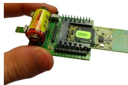
Figure 9 Example of a static node that tracks the position of the building occupant by wireless communicating with the occupant sensor
