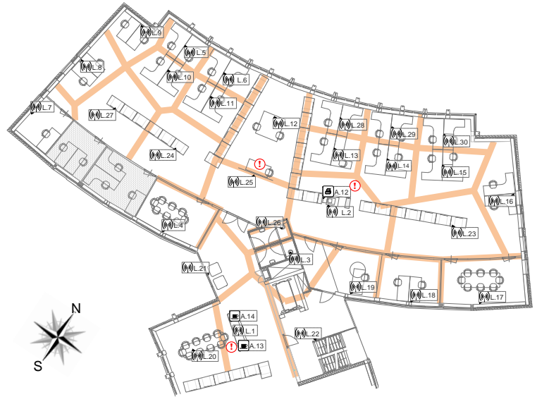
Figure 10 Positions of the static nodes creating a mesh of the zones for measuring the position of the building occupants on the floor. The transition region between the zones is marked by the broad orange line
