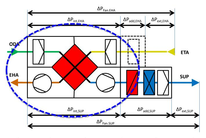
$$P_{\text{SFP}} = \frac{\Delta p_{\text{int tot}}}{\eta_{\text{tot}}} + \frac{\Delta p_{\text{add tot}}}{\eta_{\text{tot}}} + \frac{\Delta p_{\text{ext tot}}}{\eta_{\text{tot}}} = \frac{\Delta p_{\text{int stat}}}{\eta_{\text{stat}}} + \frac{\Delta p_{\text{add stat}}}{\eta_{\text{stat}}} + \frac{\Delta p_{\text{ext stat}}}{\eta_{\text{stat}}}$$
