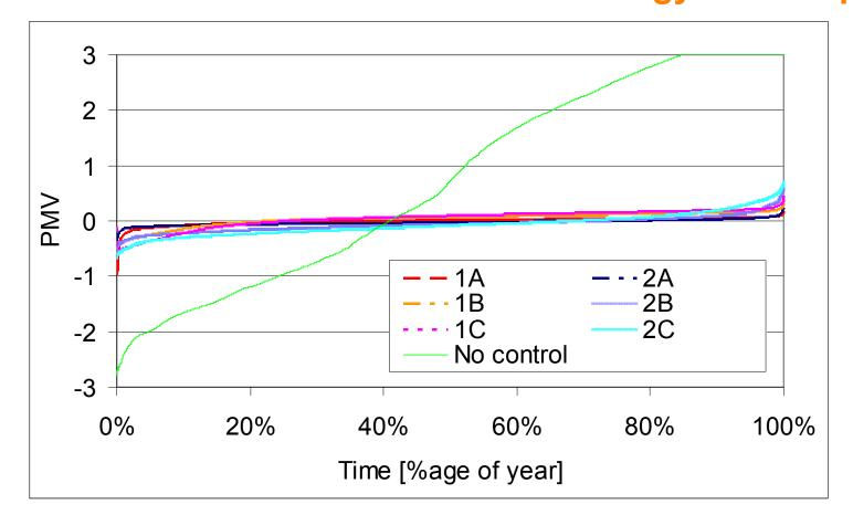
Duration curves for the PMV index in the 6 simulations and for the reference simulation. The figure shows how long time (in percentage of a year) the PMV index was below a certain value.
