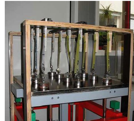
Apparatus to test alternating loads on tapes: excerpt from paper presented by T. Ackermann
