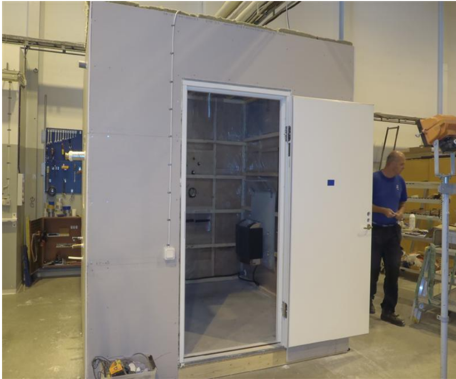
Test room for accelerated aging: excerpt from paper presented by M. Hansen
