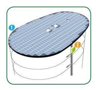
The roofing is covered with 560 m² of solar panels that ensure an annual production of 82000 kWh
