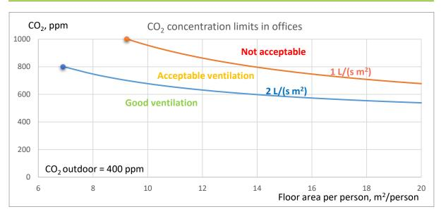
Figure 8.  $CO_2$  concentration (absolute values that include outdoor concentration) dependency on ventilation rate and occupancy in offices.
