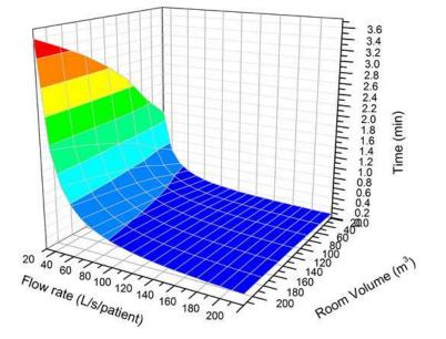
Figure 15. illustration of high airflow rates. Time to replace the air in the room as a function of airflow rate and room volume.
