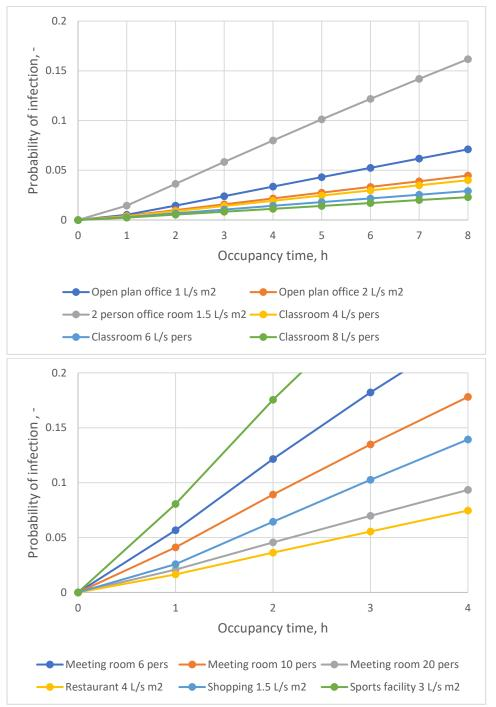
Figure 6. Infection risk assessment for some common non-residential rooms and ventilation rates calculated with the REHVA COVID-19 ventilation calculator. 1.5 L/s per m2 ventilation rate is used in 2 person office room of 16 m2, and 4 L/s per m2 in meeting rooms. Detailed input data is reported in Table 3.
