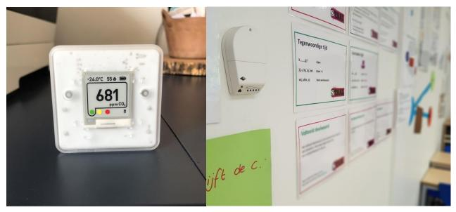
Figure 17. Examples of CO2 monitors with traffic light indicator showing the indoor air quality.
