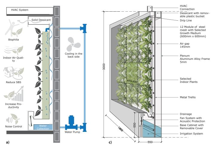
**Figure 3.** Prototype. **a)** Diagram of the LWS Design, **b)** LWS scaled Prototype and Data logger location, **c)** Section. (Armijos Moya, 2016)
