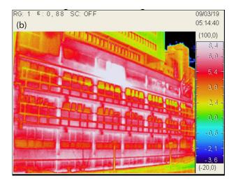
**Figure 1.** (a) VUmc Policlinic building. (b) A thermal picture of policlinic's façade highlighting, as bright patterns, the several thermal bridges within the envelope.
