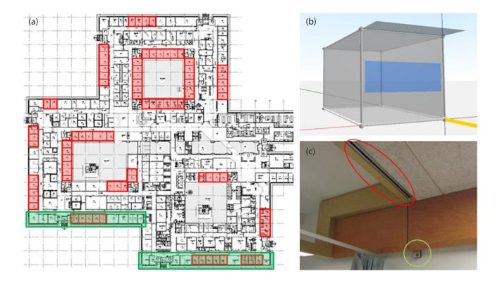
**Figure 3.** (a) Plan of policlinic building with highlighting of modelled space (red) and western façades (green). (b) VABI Elements<sup>©</sup> model. (c) Local re-heating system: air inlet (red) and temperature set-point control (green).
