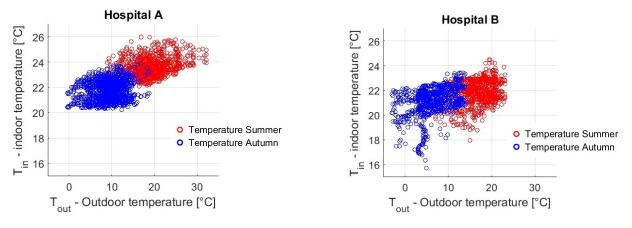
**Figure 4.** Comparison between indoor and outdoor temperature for hospital A (a) and hospital B (b) based on mean hourly data of all measured rooms.
