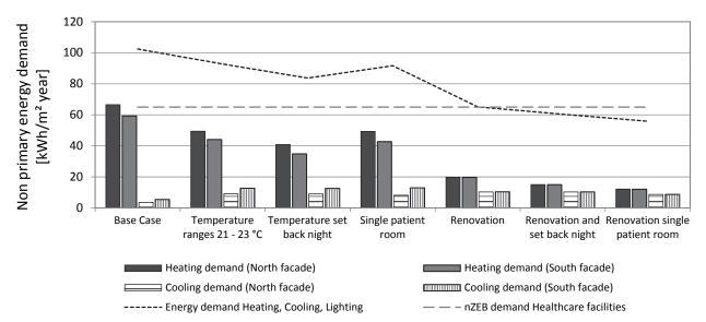
**Figure 5.** Heating and cooling demand per square meter for different scenarios with heating and cooling set-point of  $23-25^{\circ}$ C for the base case and  $21-23^{\circ}$ C for the other scenarios. For the scenarios with temperature set back, heating set point is  $18^{\circ}$ C during the night (9:00 p.m. – 6:00 a.m.).
