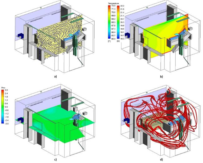
**Figure 2.** Results for the base case analysis showing a) airflow patterns, b) temperature distribution, c) PMV distribution at 4 feet (1.2 m) height, and d) resulting flow pathlines indicating probable trajectory of airborne particles released from the patient's face. This HVAC configuration entrains airborne particles back into the supply air stream which eventually spreads into the entire room.
