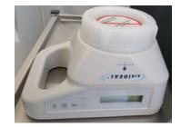
Figure 3. Measurement instruments, a) AEROTRAK<sup>™</sup> Handheld Particle Counter Model 9306, b) CFU measurement device.
