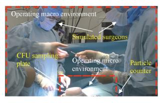
**Figure 2.** The locations of the measurement instruments for CFU measurement and particle measurement.
