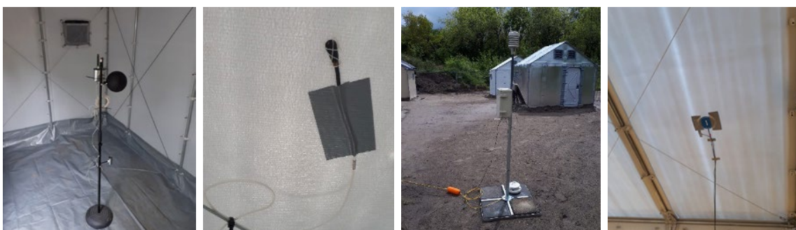
Figure 2. From left: 1. Tripod with air temperature and RH sensors and a black globe to measure the MRT. 2. Thermistor applied to the centre of a roof panel, fixated with iron wire. 3. On-site weather station. 4. Heat flux plate.
