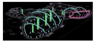
Ventilation ducts on the inner side of glass façade and displacement diffusers.
