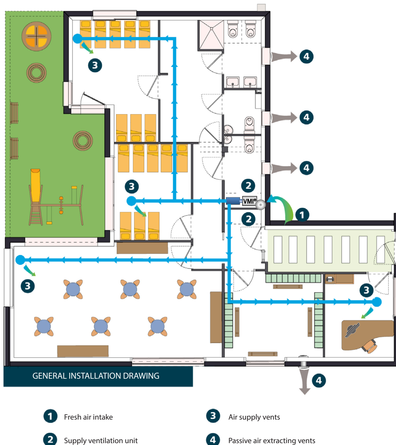
Figure 2. The fresh air taken from outside the building and after passing through the ventilation supply unit is routed through the distribution network to the various premises of the nursery. Air is evacuated outside by passive exhaust vents mounted on the windows frame.
