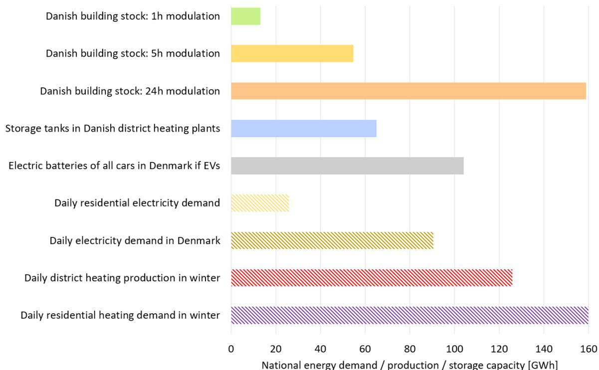
**Figure 3.** Thermal storage capacity in the indoor environment of the entire Danish building stock compared with key storage sources, energy demands and productions.
