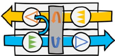
If the extract fan is placed on the extract side of the rotor, then the leakage will be in the other direction:
