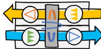
The fourth mode of leakage is from extract to supply on the room side of the rotor like this:
