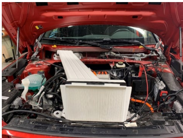
Figure 1. Pre-filter prototype installation in an existing production vehicle's thermal compartment.
