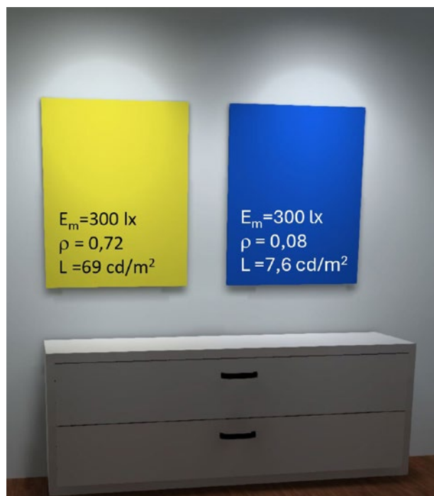
Figure 2. Luminance depends on illuminance and reflectance. For diffusing surfaces L = E \cdot \rho / \pi .
