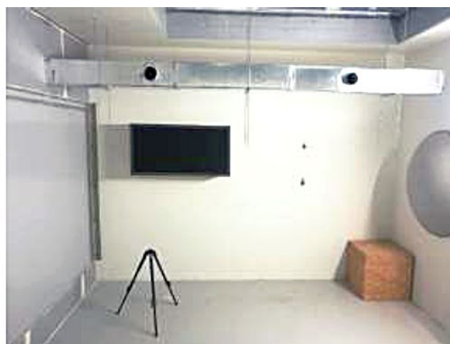
CLIMAVER® A2 NETO 25 mm ductwork with 2 openings ( \phi = 125 mm) at 1 m and 3 m from the separating wall in both rooms, left: source room, right: receiving room.
