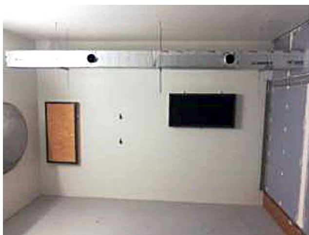
CLIMAVER® A2 NETO 25 mm ductwork with 2 openings ( \phi = 125 mm) at 1 m and 3 m from the separating wall in both rooms, left: source room, right: receiving room.
