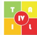
Fig. 1. The TAIL rating scheme with four colours representing the quality levels of each IEQ component and the overall IEQ level; the colours are just examples of the quality levels, and each of the TAIL components can have any of the four quality levels represented by four colours. The Roman numeral in the centre shows the integrated overall quality level determined based on the quality level of the four components of TAIL.
