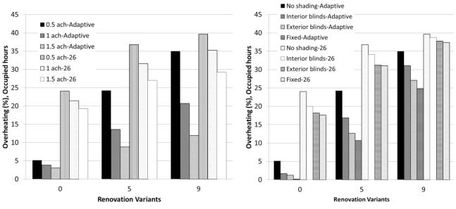
**Figure 4.** Percentage of overheating hours (measured only for occupied hours) for different renovation variants (Table 2), methods, ventilation rates and shading systems, for the southern French case study.
