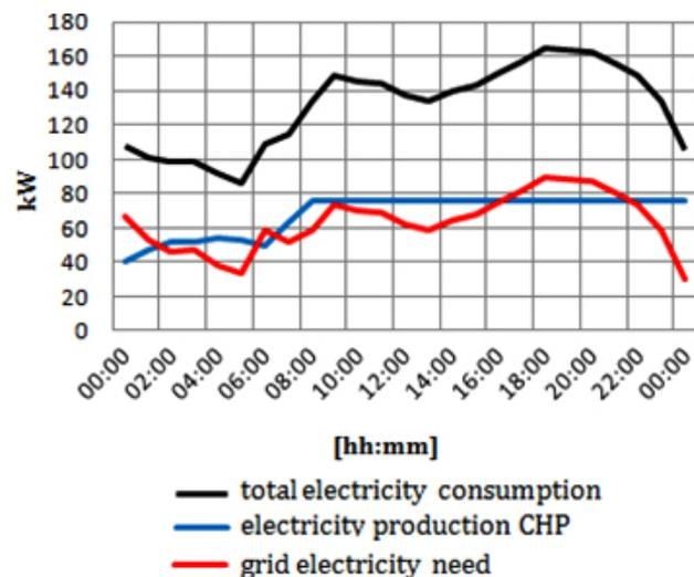
**Figure 3.** Expected typical daily electricity flow pattern.
