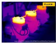
Figure 10. Bad connections caused the temperature of the cables to be above 70°C. This is above the limit recommended by European Committee for Electrotechnical Standarization – CENELEC HD 516 for PVC cables.
