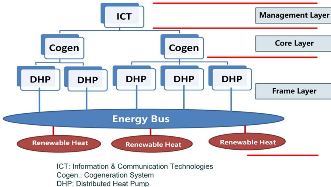
Figure 1. Three levels of Smart Micro Energy Network (SMEN).
