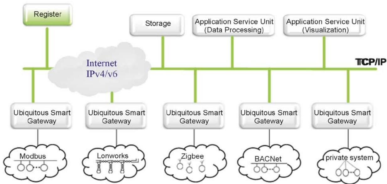
**Figure 6.** Systematic network architecture of IEEE 1888.
