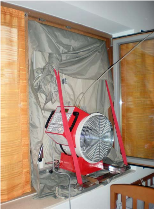
Figure 4. Blower Door test.
