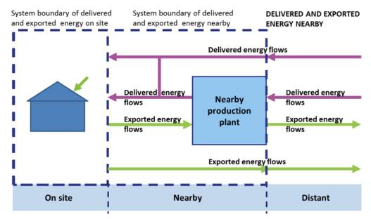
Figure 2. REHVA definition provides for nearby production invested by the building owner an equal treatment compared to on site production. There are no technology limitations, a public grid or district heating or cooling networks can be also used to connect a new renewable energy capacity to the building and to utilize with a primary energy factor related to this new capacity.
