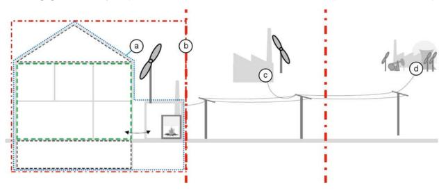
**Figure 1.** prEN15603:2013 defines energy balance of a building (a), on site perimeter (b), nearby (c) and distant energy production (d).
