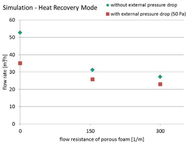
**Figure 5.** Flow rates of the heat recovery mode at different flow resistance loss coefficients for the porous elements without external pressure (green) and with an external pressure of 50 Pa (red) at each in-/outlet.
