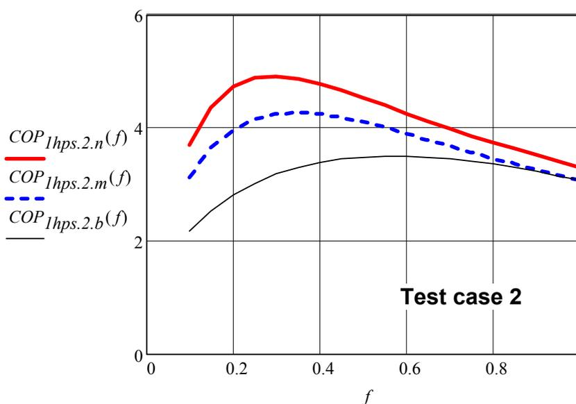
Figure 7. The coefficient of performance of the heat pump system ( $COP_{hps}$ ) as function of the fractional capacity ( $0 \leq f \leq 1$ ) for three alternative motor topologies. Powers to the evaporator and condenser fans are constant.
