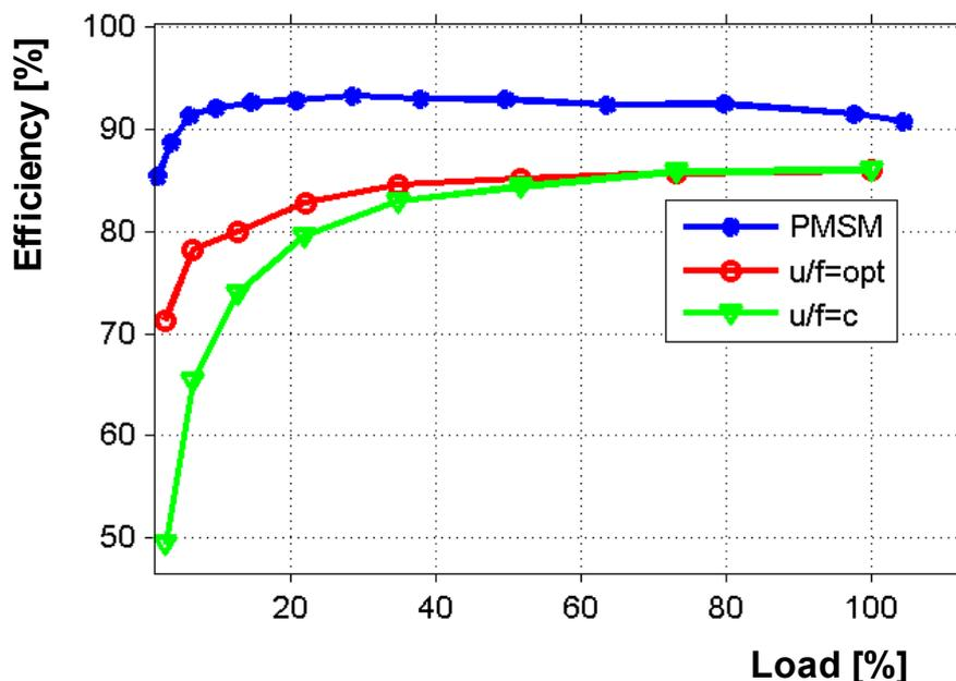
**Figure 5.** Comparison by Åström<sup>[25]</sup> of three alternative motor configurations. The two lower represent current practices and the top curve represent a new PMSM motor developed by Åström.
