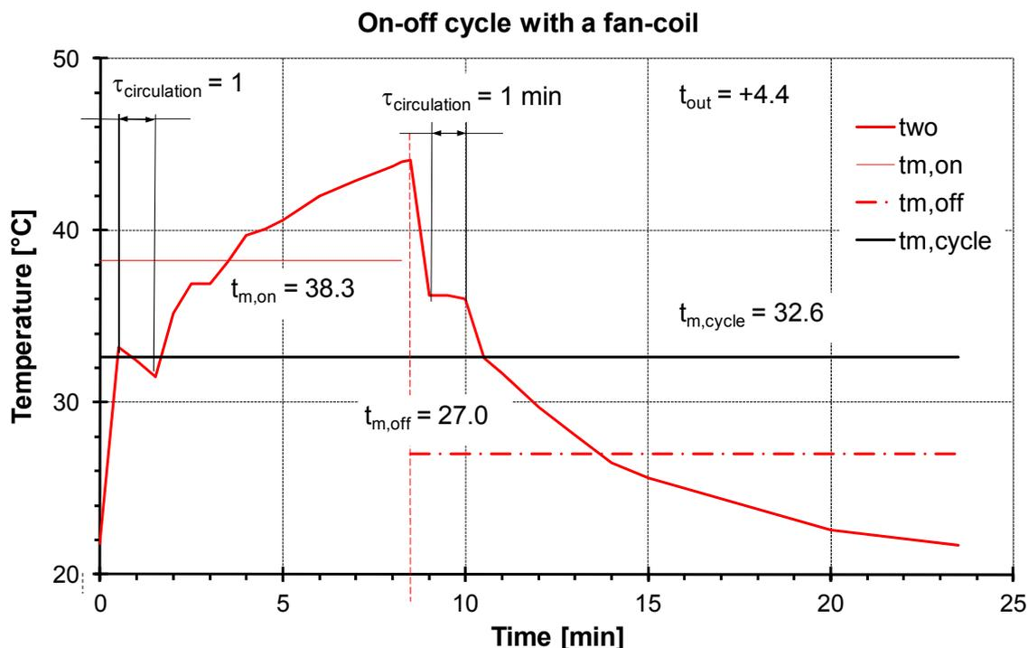
**Figure 2. One complete on-off cycle with a heat pump connected to a combined radiator and fan-coil system (Fahlén<sup>[9]</sup>).**
