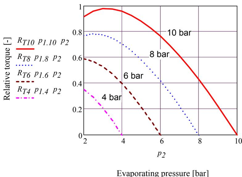
Figure 4. Relative torque  $T = T_{com} / T_{com,0}$  as function of evaporating pressure  $p_2$  with  $p_1 = p_{1,0} = 10$  bar,  $p_{2,0} = 2$  bar (based on an example according to Fahlén with an air-to-air heat pump and propane, R290, as refrigerant:  $t_{1,0} = 29$  °C,  $p_{1,0} = 10.5$  bar and  $t_{2,0} = -3$  °C,  $p_{2,0} = 4.3$  bar).
