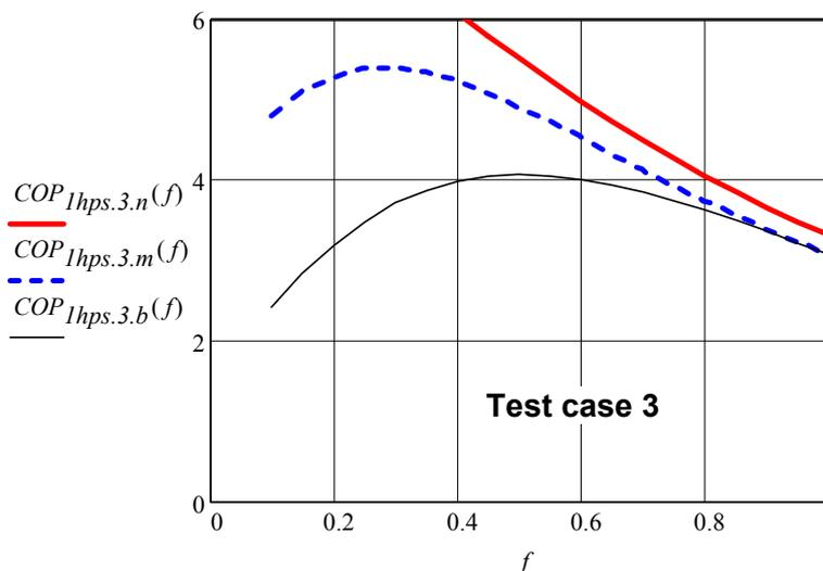
Figure 8. Coefficient of performance of the heat pump system ( $COP_{hps}$ ) as function of the fractional capacity ( $0 \leq f \leq 1$ ) for three motor topologies. Evaporator and condenser fan powers vary in relation to the relative thermal capacity.
