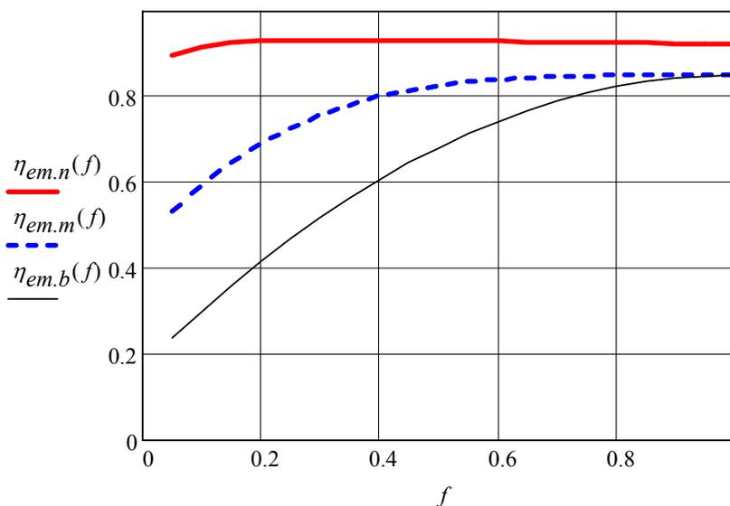
Figure 6. Motor efficiency ( $\eta_{em}$ ) as a function of the fractional capacity ( $f$ ). Index  $b$  represents a base case with today’s standard practice,  $m$  corresponds to modern, state-of-the-art equipment and  $n$  is our newly developed concept (motor power around 1 kW).
