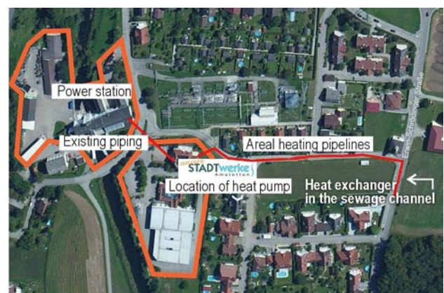
Figure 3. The municipality of Amstetten, as one of the suitable locations, has been the first to realize the concrete implementation. 400 single-family homes can be heated now all over the year with the heat pump.
