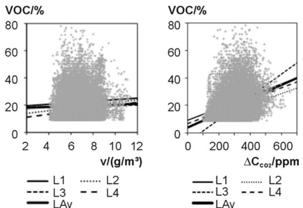
Professor **Dennis Johansson** from Lund University presented the response of a mixed gas sensor. The measured mixed gas sensor output is shown as a function of indoor vapour content for all measured points in all 4 buildings in the left, and as a function of difference in CO<sub>2</sub> concentration between indoor and outdoor in the right.
