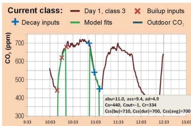
An example of ventilation analysis for a class. Red markers = build-up phase; blue markers = decay phase; green lines = ventilation model fit. Decay estimate (4.9 h<sup>-1</sup>) is lower than build-up (11 h<sup>-1</sup>) as the demand control adjusts the ventilation according to the CO<sub>2</sub>-level monitored in the ventilation system.
