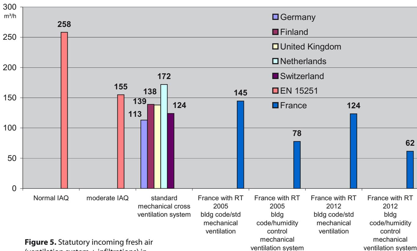
**Figure 5.** Statutory incoming fresh air (ventilation system + infiltrations) in different European countries compared to EN standard.
