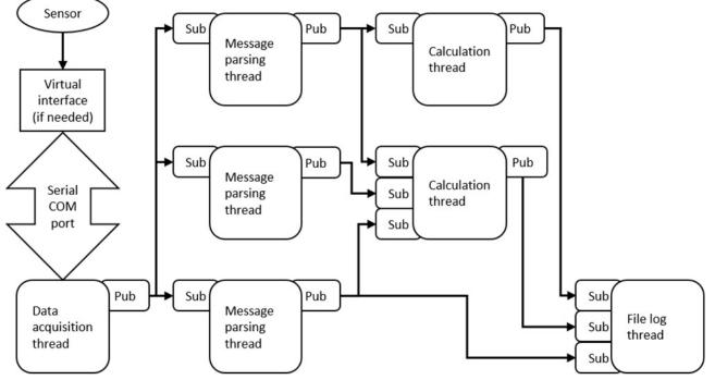
Figure 4. Data handling Volkerak software structure.
