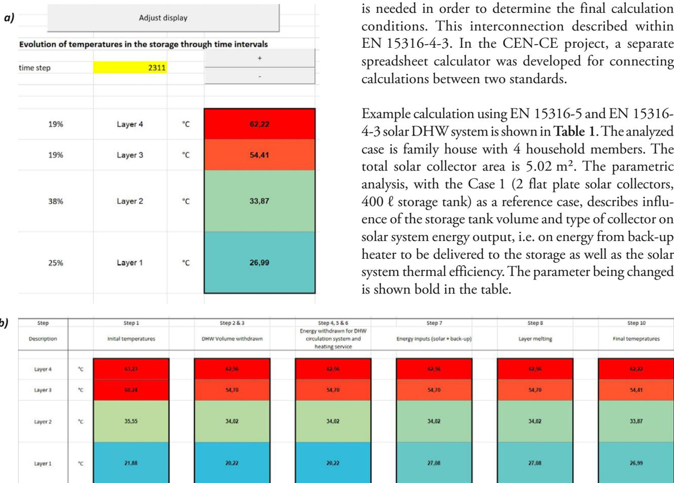
Figure 4. a) Storage tank temperatures in a chosen hour; b) Insight of each calculation step temperature stratification).
