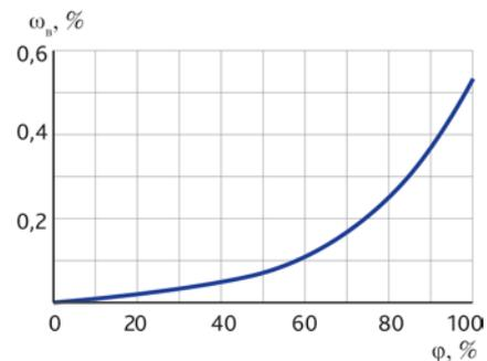
Figure 2. Water vapor sorption isotherm for regular brick.
