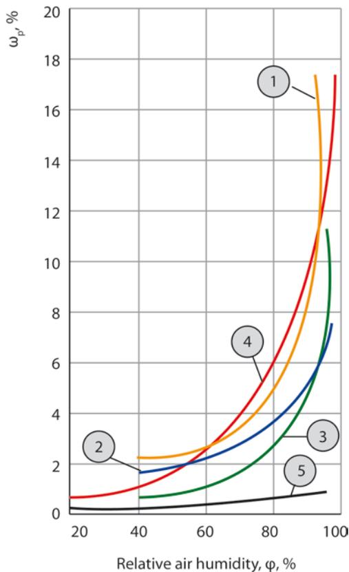
**Figure 3.** Sorption isotherms for red brick samples.
