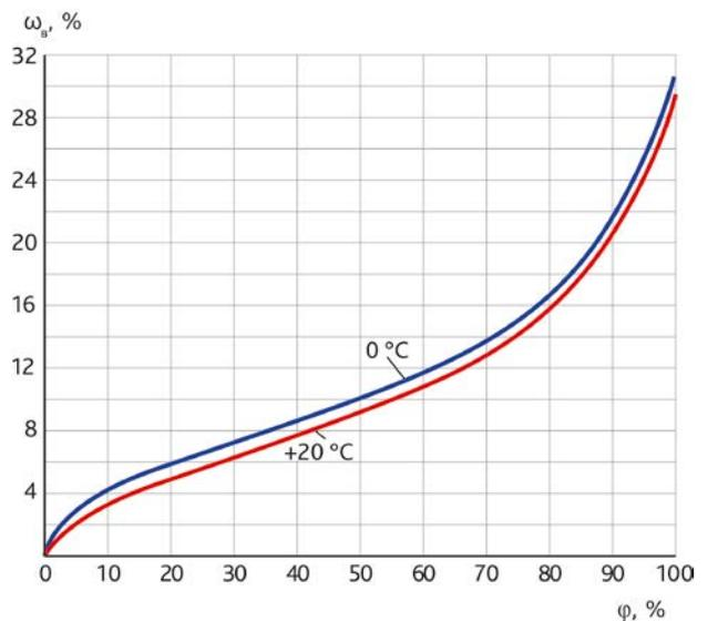
Figure 1. Water vapor sorption isotherm for wood.
