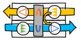
This leakage will depend on the pressure difference between the extract and the supply and if the fans are correctly positioned as shown, can be eliminated by throttling the extract air so that the pressure difference is in the right direction. This extra pressure drop must be included in the exhaust fan.
