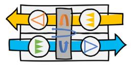
4. Leakage from extract to supply on the room side of the rotor
