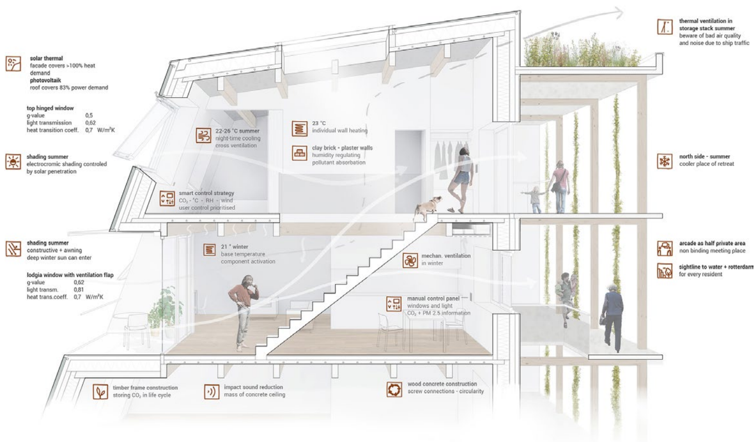
Figure 4. Section through one of the maisonette apartments; visualization of the heating, ventilation and smart control strategy.
