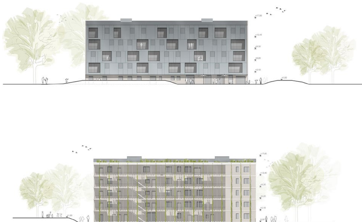
Figure 2. South elevation (top): tilted facade with solar thermal collectors and loggias; North elevation (bottom) with wooden arcade and green roof.
